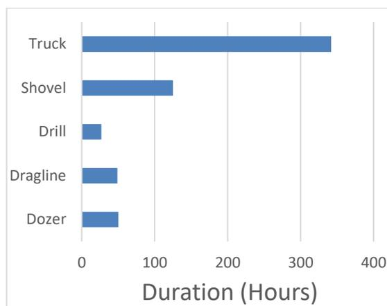
**Figure 71: Operational Downtime by Equipment Type – September 2021**
