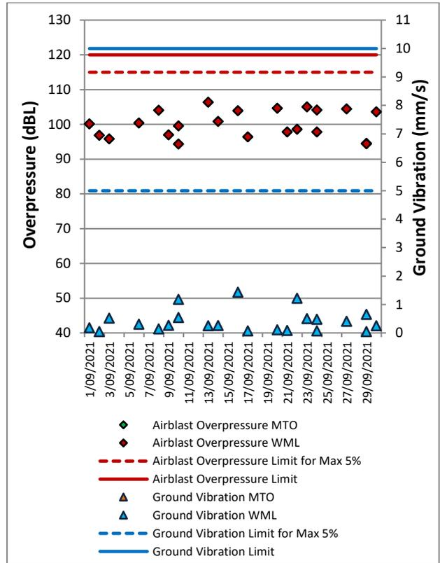
Figure 67: Wambo Road Blast Monitoring Results – September 2021
