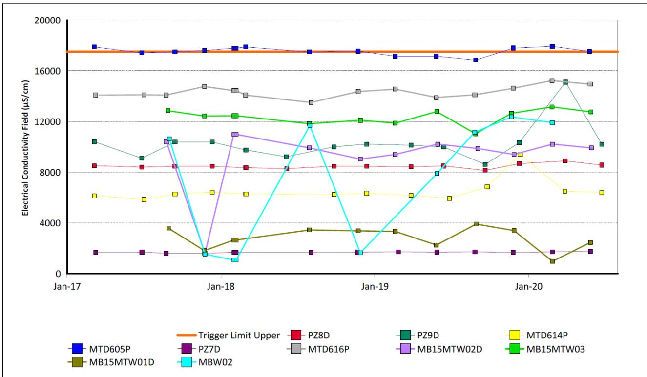
Figure 28: Shallow Overburden Electrical Conductivity Trend – June 2020
