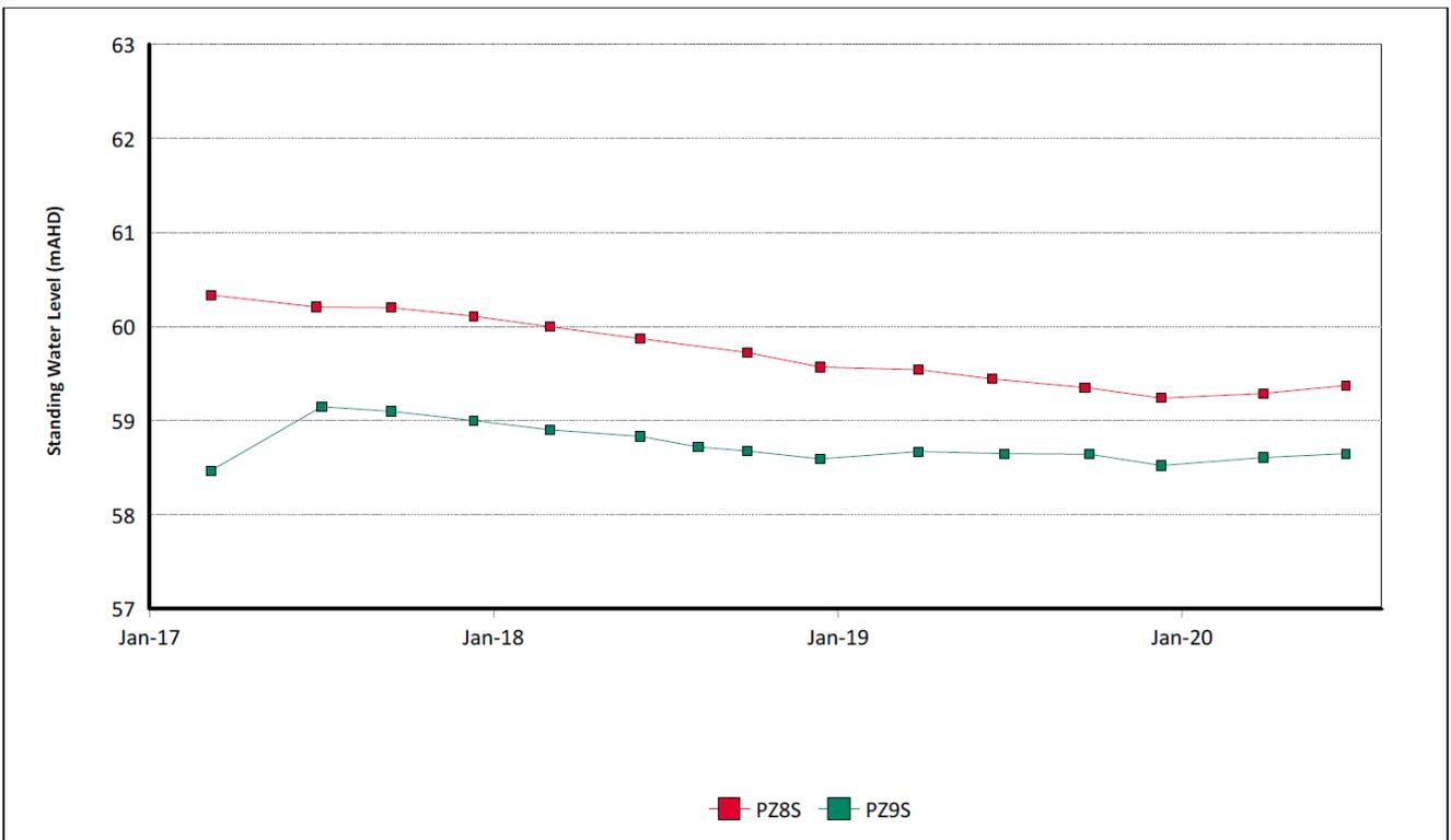
Figure 44: Wollombi Alluvium Standing Water Level Trend – June 2020
