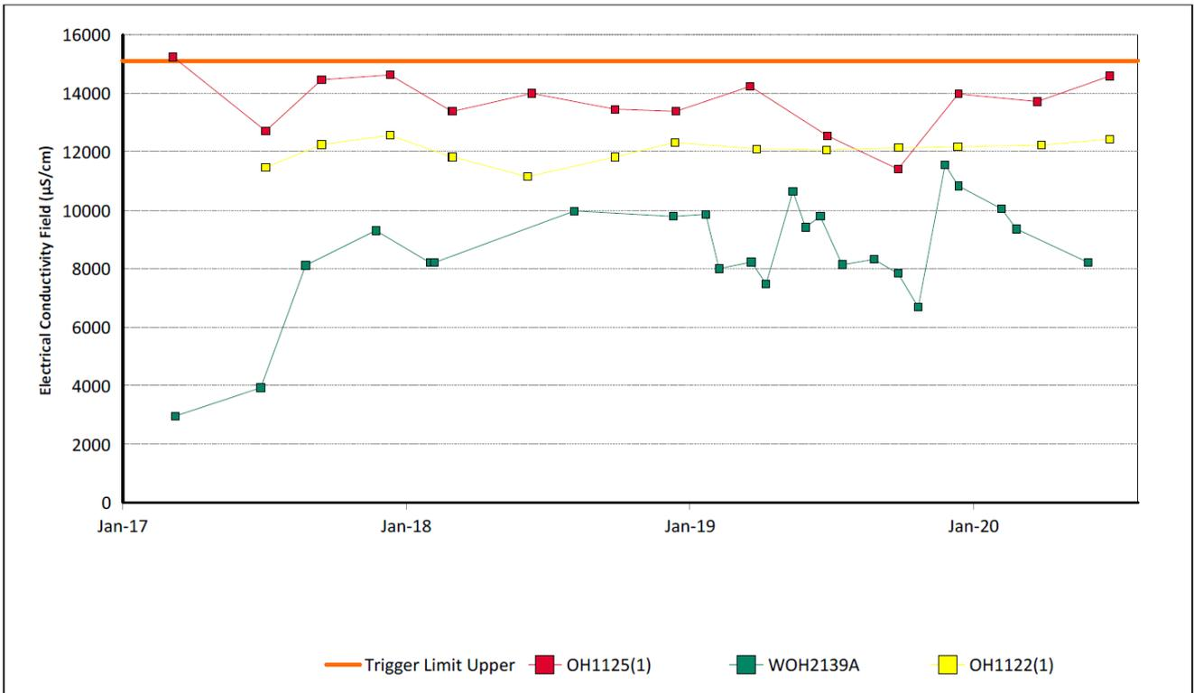
Figure 19: Blakefield Seam Electrical Conductivity Trend – June 2020
