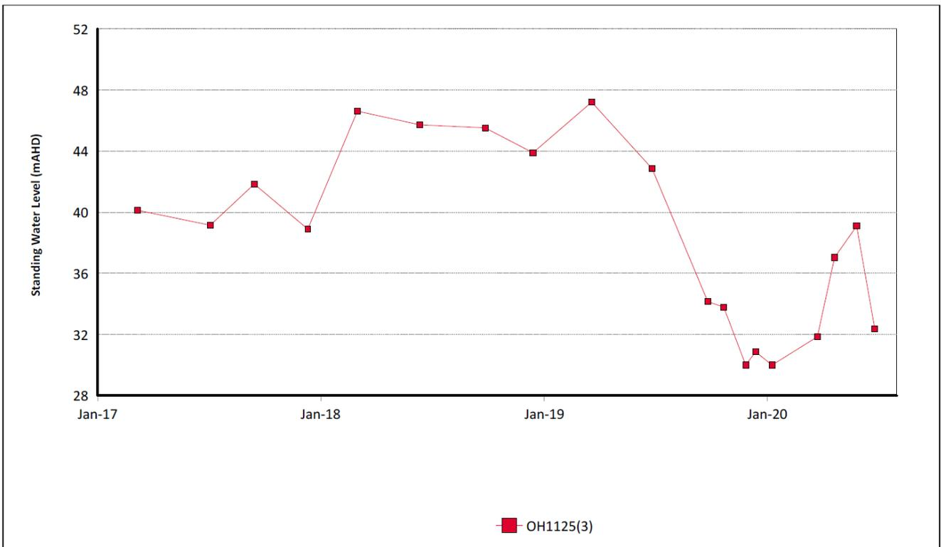
Figure 24: Bowfield Seam Standing Water Level Trend – June 2020
