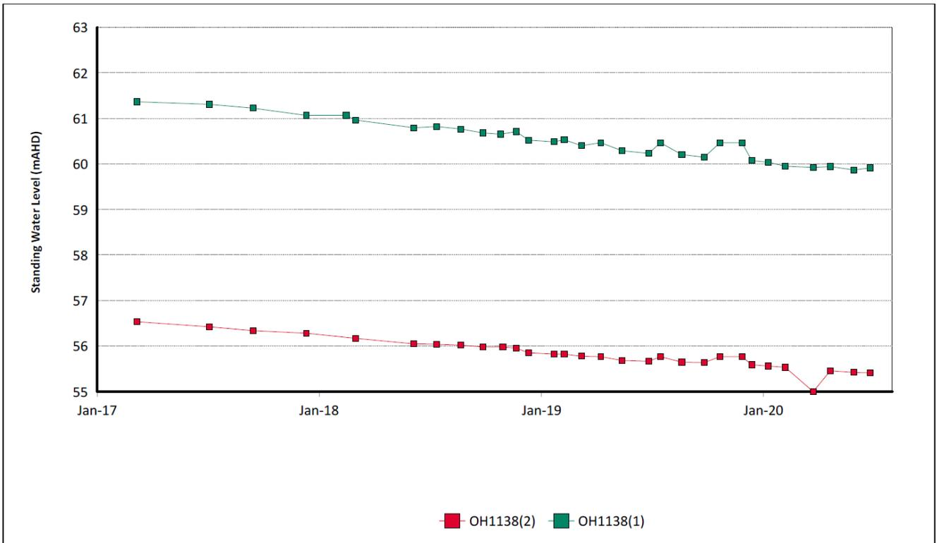
Figure 39: Warkworth Seam Standing Water Level Trend – June 2020
