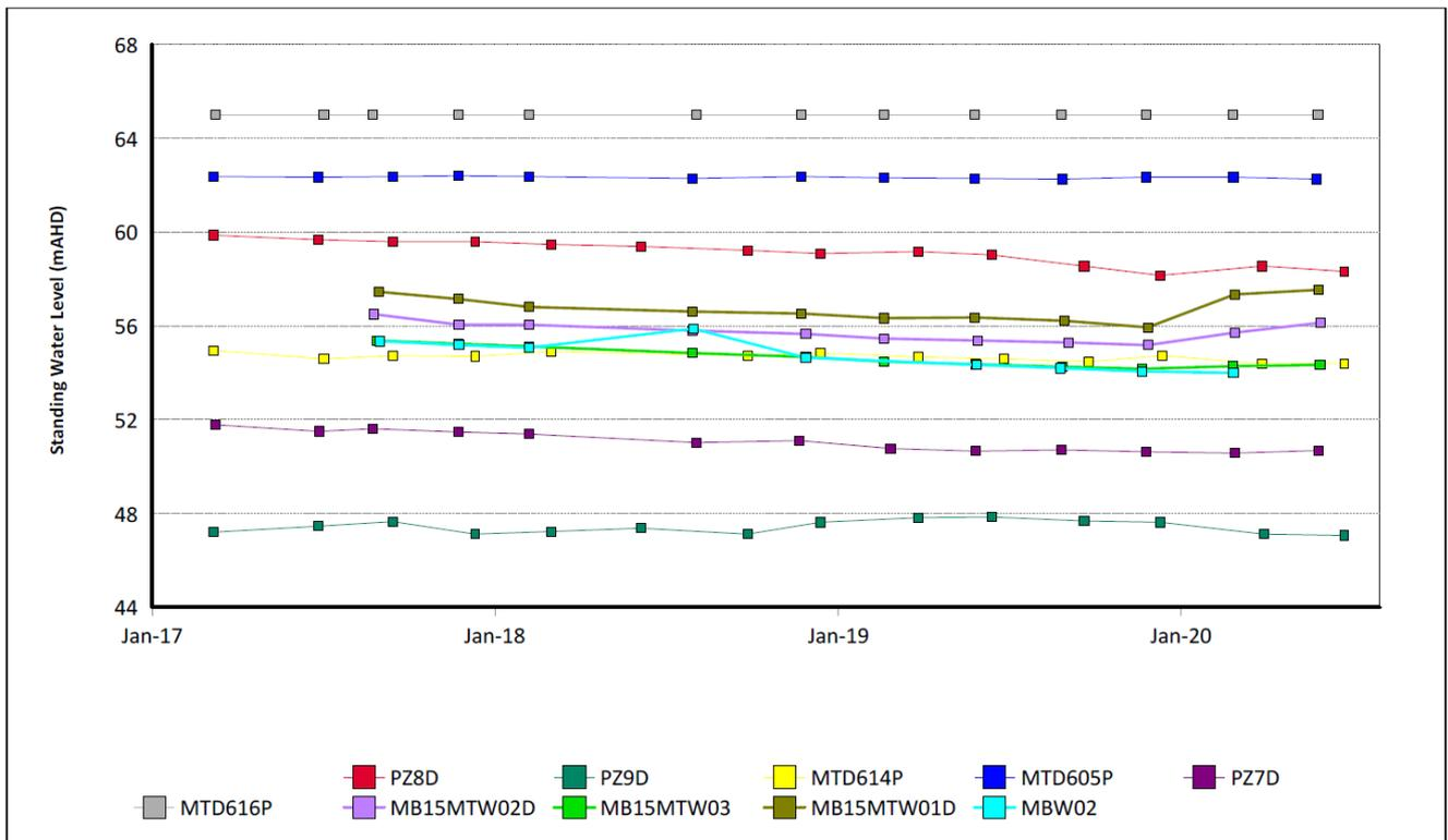
Figure 30: Shallow Overburden Standing Water Level Trend – June 2020
