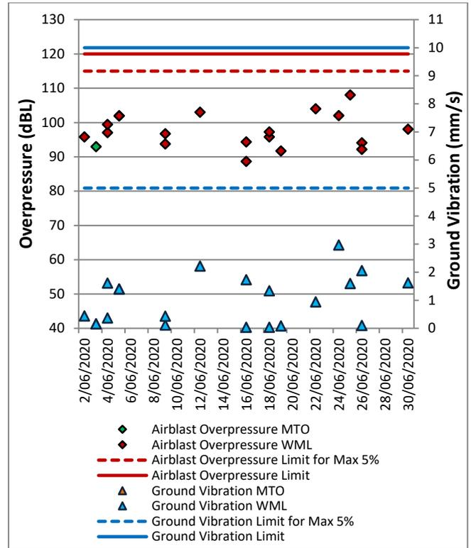
Figure 67: Wambo Road Blast Monitoring Results – June 2020
