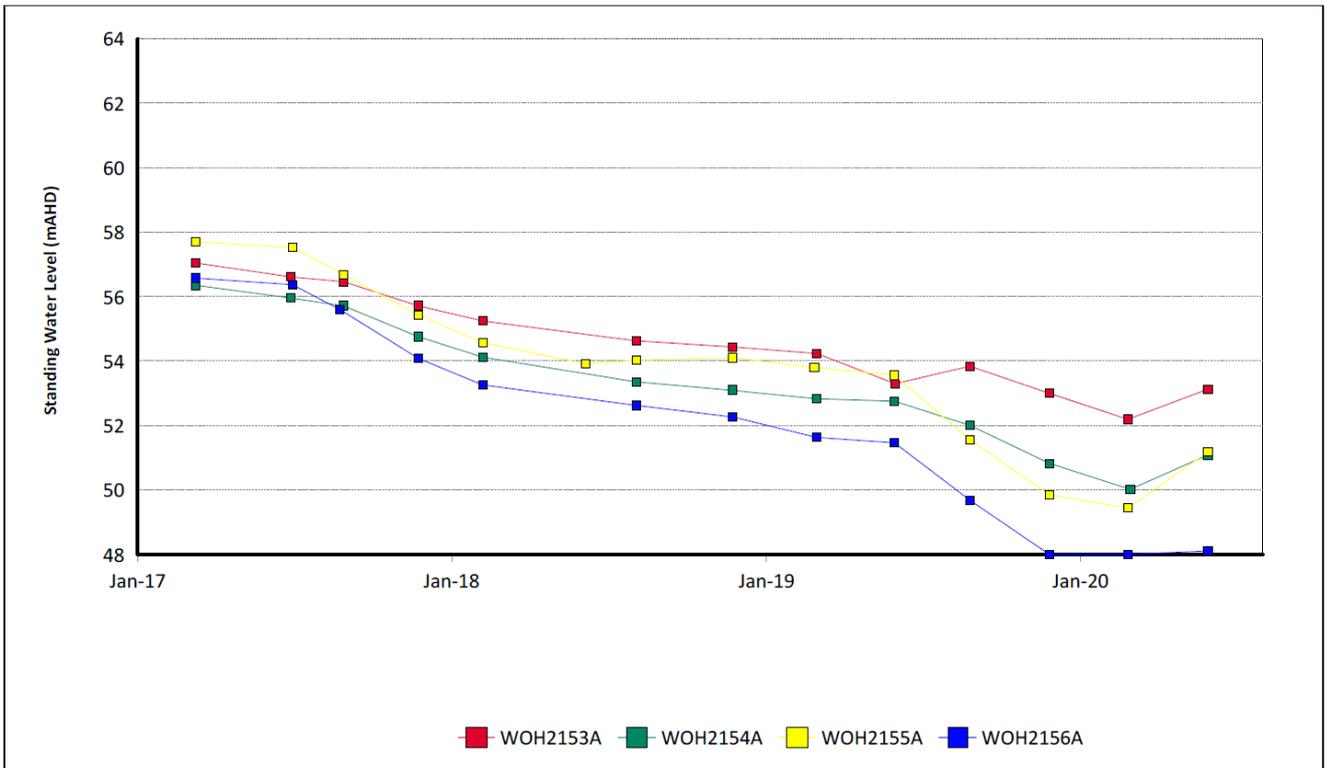
Figure 27: Redbank Seam Standing Water Level Trend – June 2020
