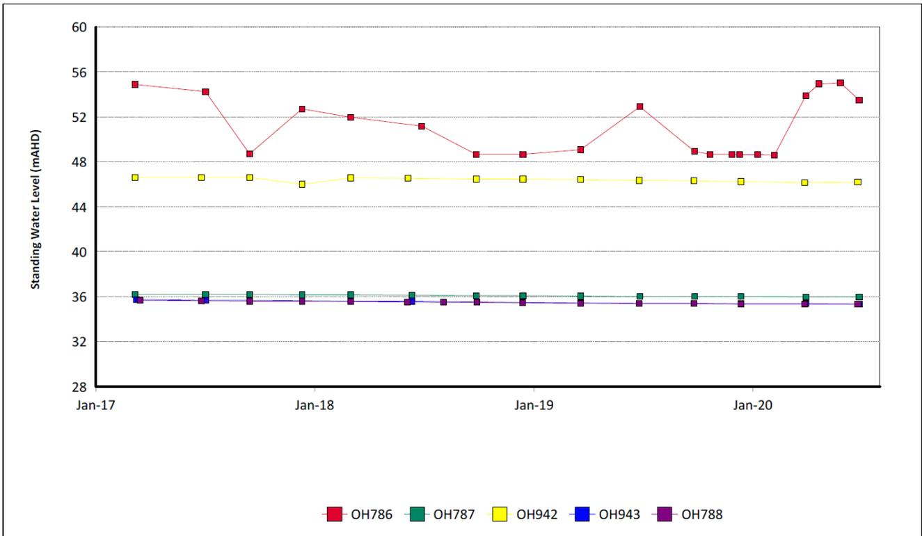
Figure 61: Hunter River Alluvium Standing Water Level Trend – June 2020
