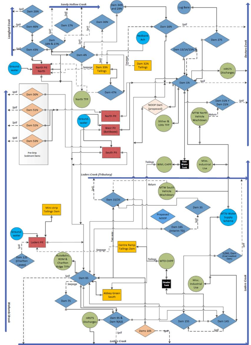
Figure 3 – MTW Water Management System Schematic
