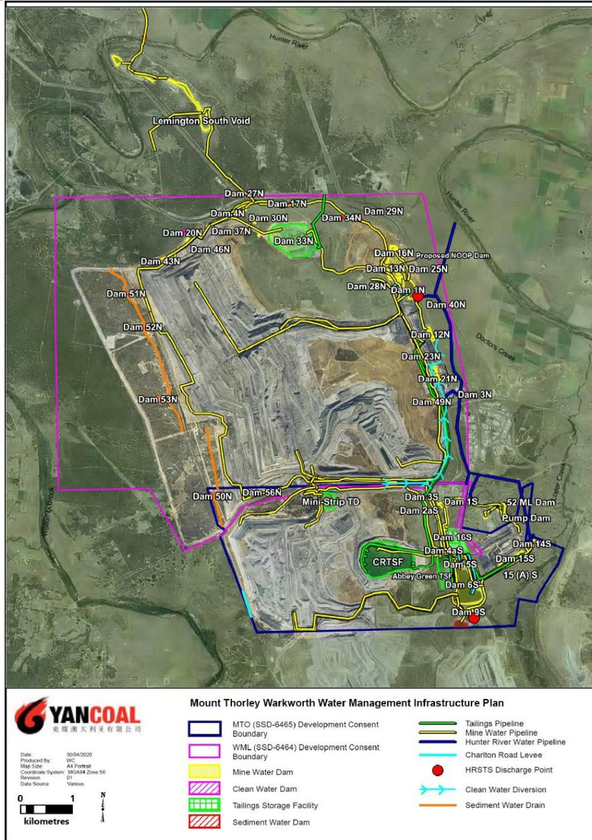
Figure 2 – MTW Water Management Infrastructure Plan
