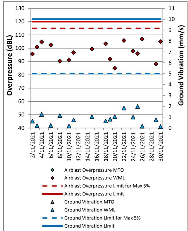
Figure 14: Warkworth Blast Monitoring Results – November 2021
