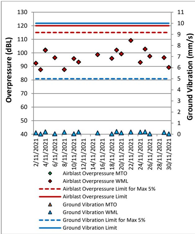
Figure 11: MTIE Blast Monitoring Results – November 2021
