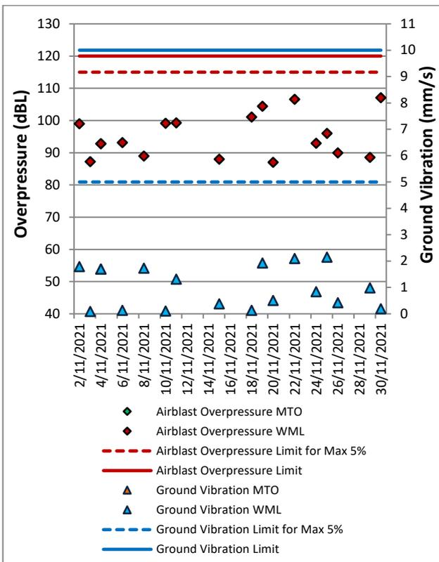
Figure 12: Wollemi Peak Road Blast Monitoring Results – November 2021
