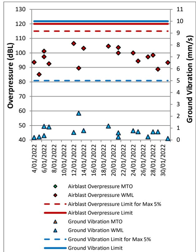
Figure 14: Warkworth Blast Monitoring Results – January 2022
