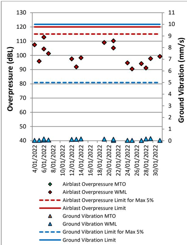
Figure 11: MTIE Blast Monitoring Results – January 2022
