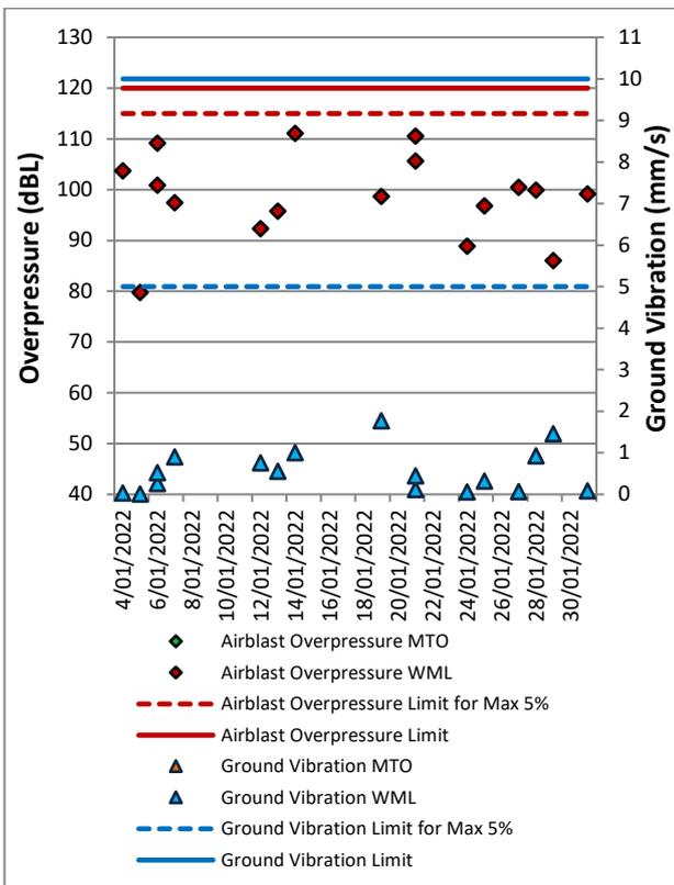
Figure 12: Wollemi Peak Road Blast Monitoring Results – January 2022
