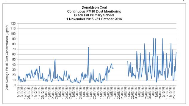
Figure 6.5 Results of Dustrak Continuous Monitoring
