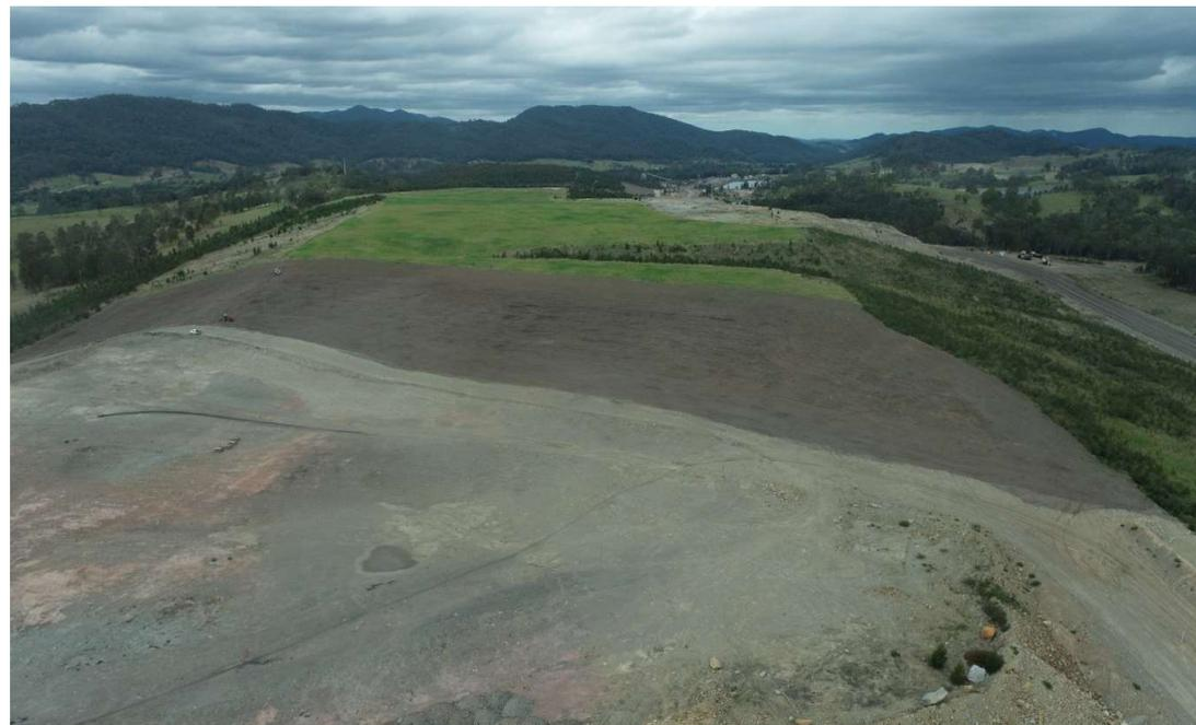
Photo: Completed bulk shaping and topsoiling at Weismantel waste emplacement, taken October 2021.
