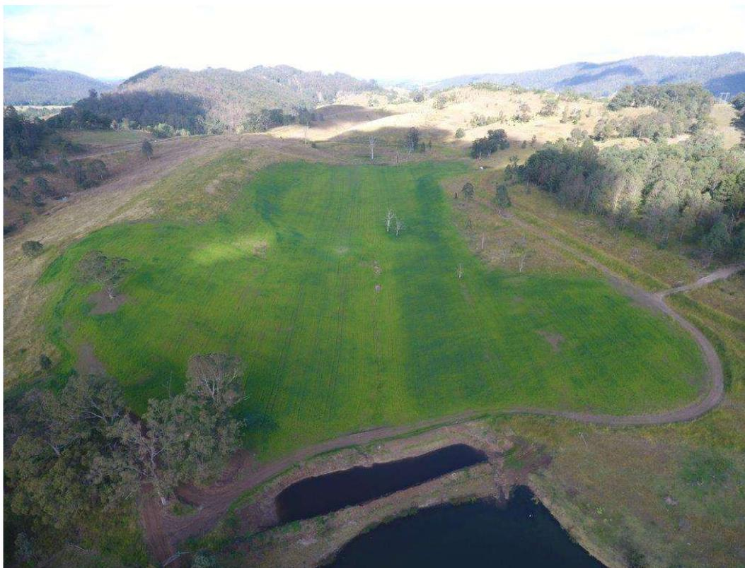
Photo: Shaping and topsoiling completed at Auxiliary Dam 1, Jul 2020.
