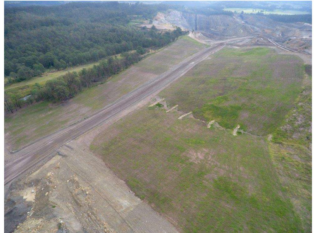
Photo: Bulk shaping and topsoiling at Weismantel waste emplacement and Duralie Haul Rd, taken Jun 2020.
