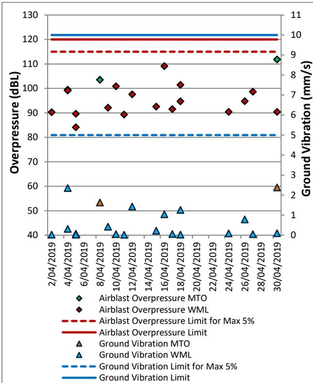
Figure 12: Wollemi Peak Road Blast Monitoring Results – April 2019
