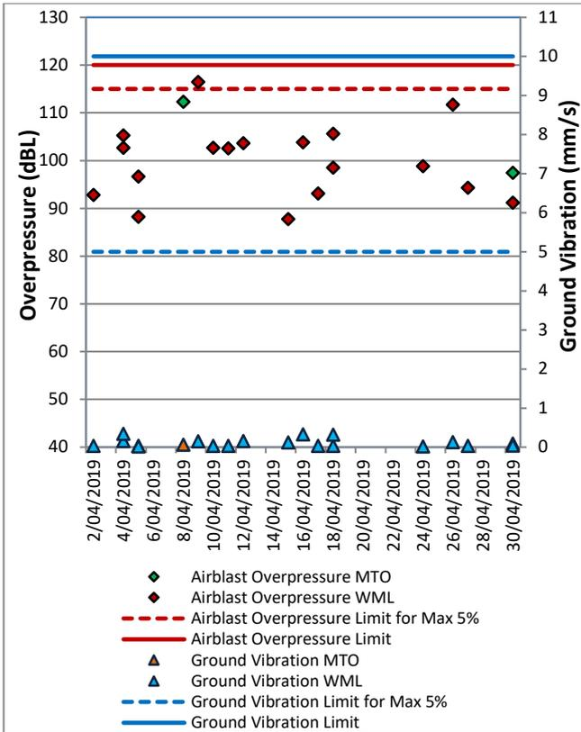
Figure 11: MTIE Blast Monitoring Results – April 2019
