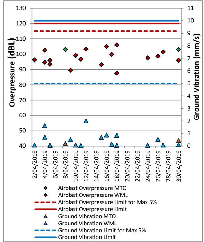
Figure 13: Wambo Road Blast Monitoring Results – April 2019
