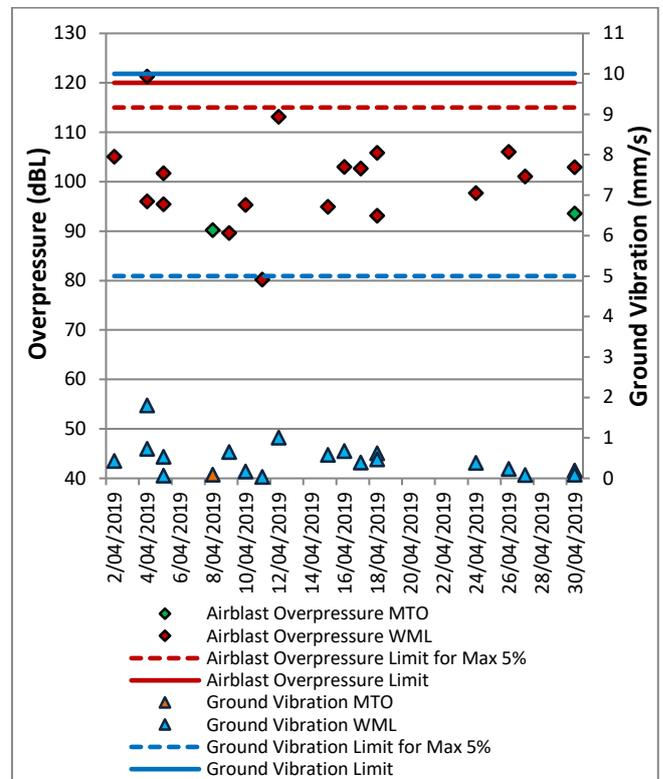
Figure 14: Warkworth Blast Monitoring Results – April 2019
