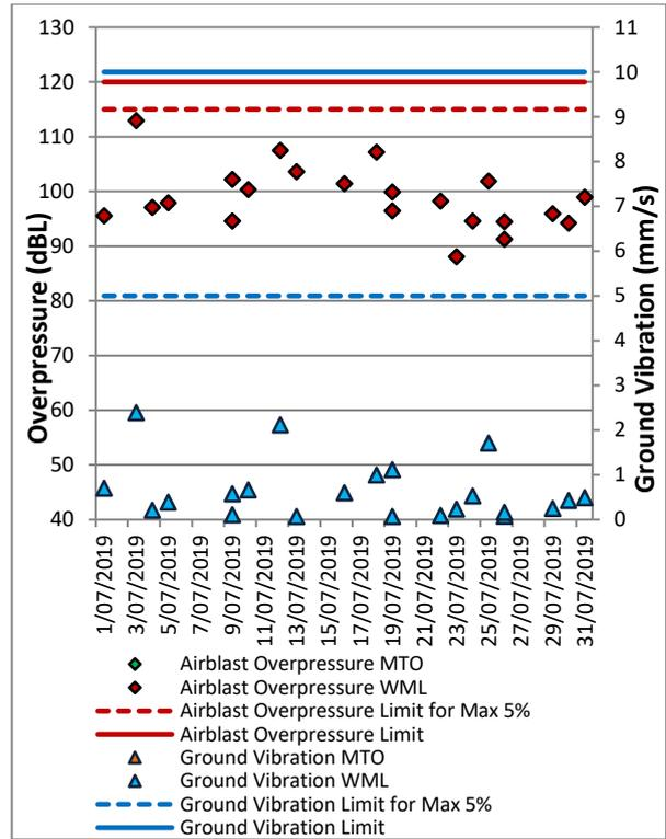
Figure 13: Wambo Road Blast Monitoring Results –July 2019
