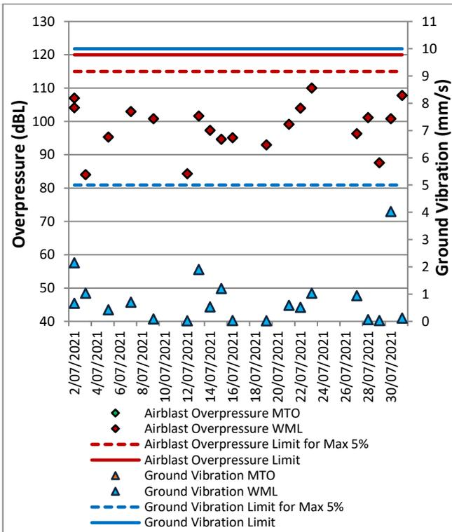
Figure 12: Wollemi Peak Road Blast Monitoring Results – July 2021
