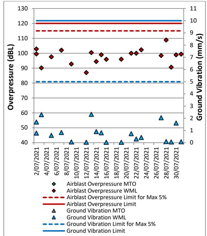
Figure 13: Wambo Road Blast Monitoring Results – July 2021
