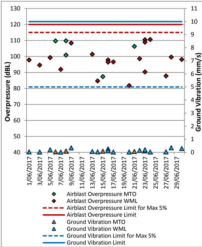
**Figure 62: MTIE Blast Monitoring Results – June 2017**
