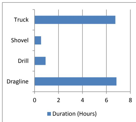
**Figure 68: Operational Downtime by Equipment Type – June 2017**
