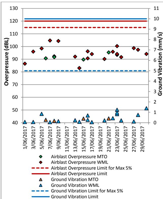
**Figure 63: Warkworth Blast Monitoring Results - June 2017**
