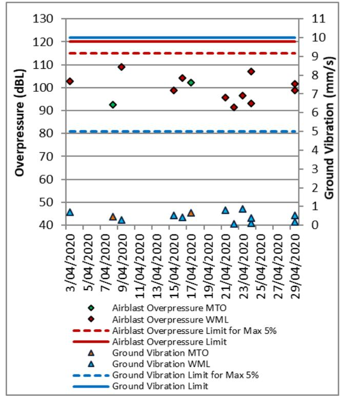
Figure 13: Wambo Road Blast Monitoring Results – April 2020
