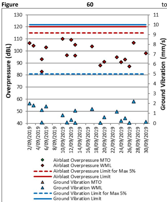
Figure 65 show the blast monitoring results for the reporting period against the impact assessment criteria. The criteria are summarised in **Table 4**.
