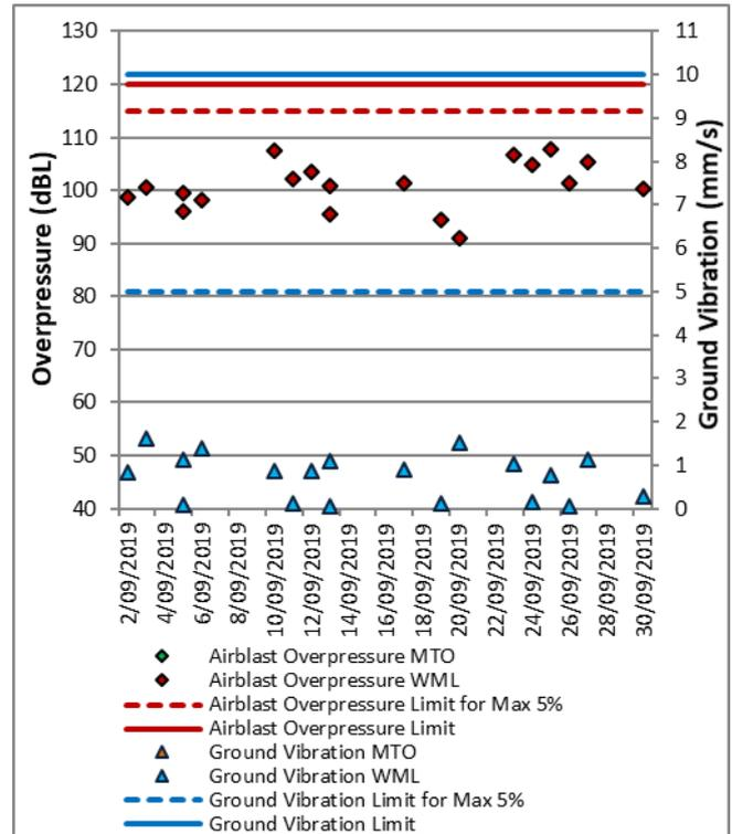
Figure 64: Wambo Road Blast Monitoring Results – September 2019
