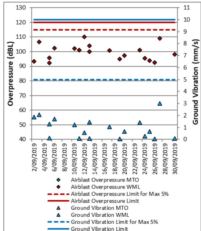
Figure 61: Bulga Village Blast Monitoring Results – September 2019
