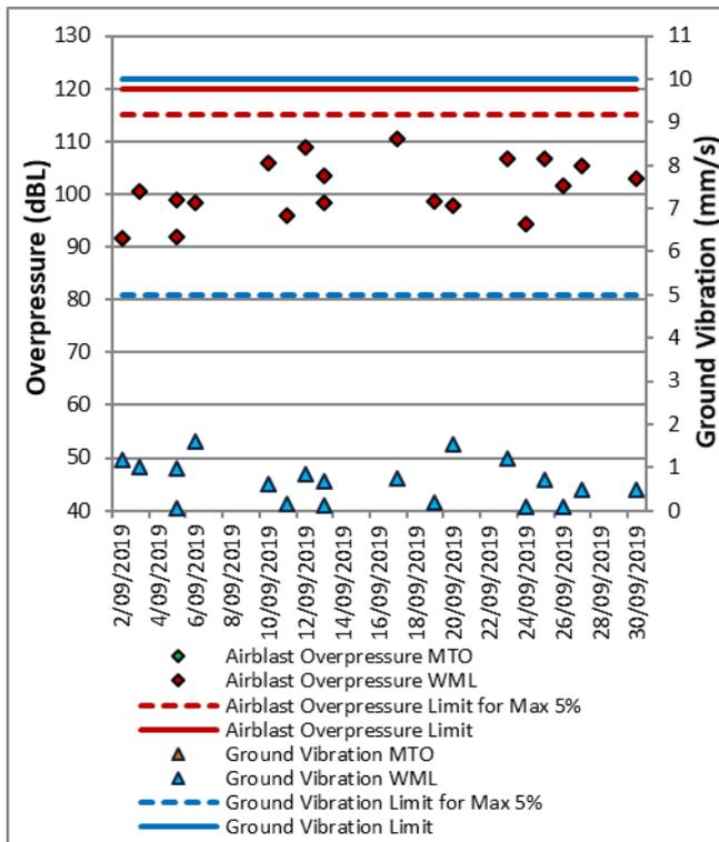
Figure 63: Warkworth Blast Monitoring Results - September 2019
