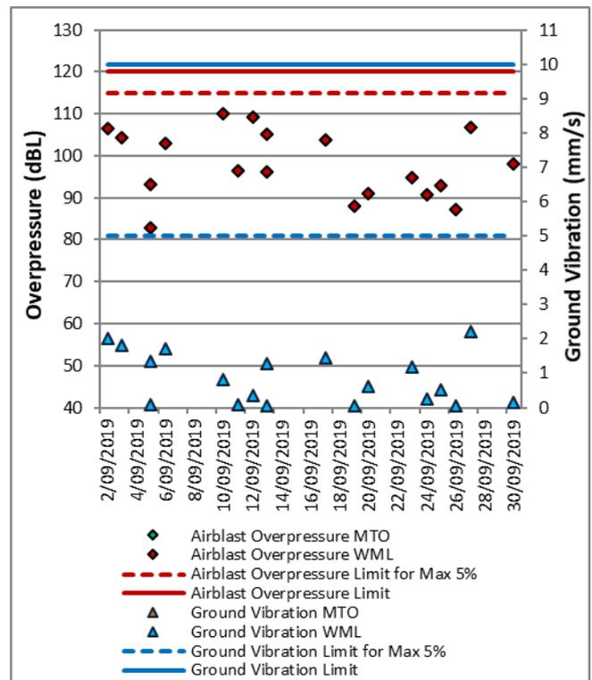
Figure 65: Wollemi Peak Road Blast Monitoring Results - September 2019
