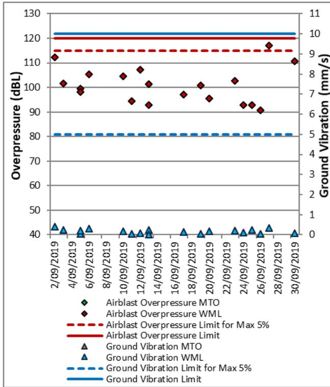
Figure 62: MTIE Blast Monitoring Results – September 2019
