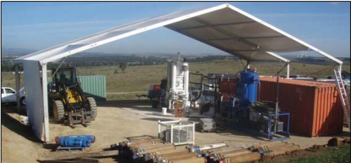
**Photograph 2: Typical raise bore drilling rig and temporary marquee**
