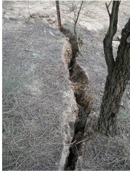
Fig. 4.7 Isolated Surface Cracking above multi-seam longwall extraction at Blakefield South Mine in the Hunter Coalfield around 200m cover
