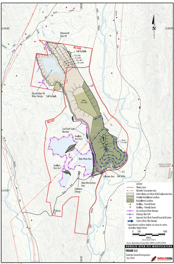
Revised waste rock emplacement design, resulting from the proposed changes to the open pits and a revision to the waste rock swell factor (i.e. the increase in volume of a tonne of waste rock in an emplacement relative to its *in situ* volume) assumed for the DEP, has determined an increase in the currently approved waste rock emplacement elevation is required to accommodate the waste rock to be mined over the remaining life of the DCM (incorporating the Modification).
