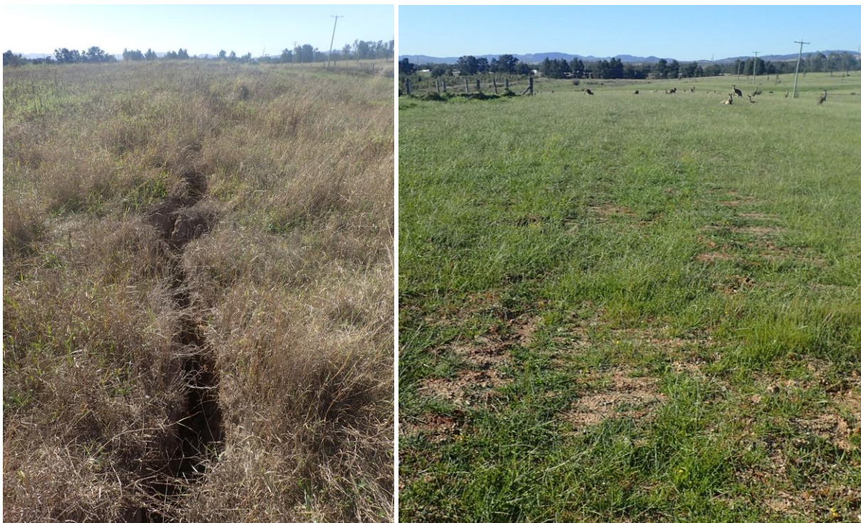
Photo 2: Example of subsidence cracking along stacked goaf edge and after crack remediation at the AUM
